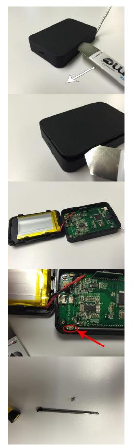
Step 1. Place a hard, thin object (letter opener, credit card, etc.) into the middle left side of the TireMinder TM66's rear case. Gently slide towards the corner of the case.
